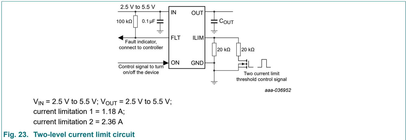
Fig. 23. Two-level current limit circuit
