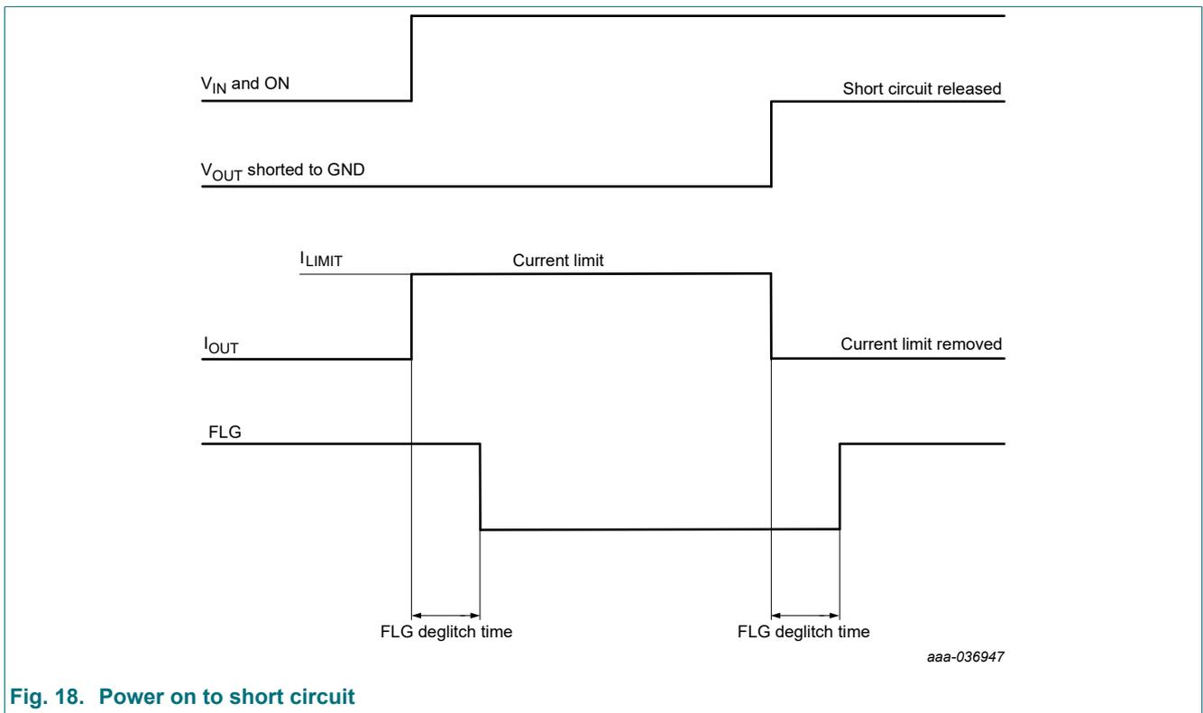
Fig. 18. Power on to short circuit
