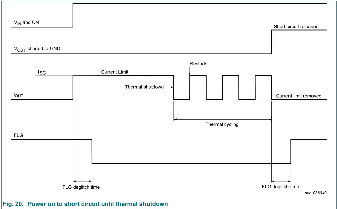
Fig. 20. Power on to short circuit until thermal shutdown
