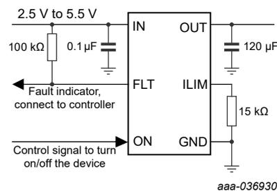
**Note:** Connect at least 120 μF capacitor at output for USB port application, other applications except USB choose output capacitor according to actual transient requirements.
