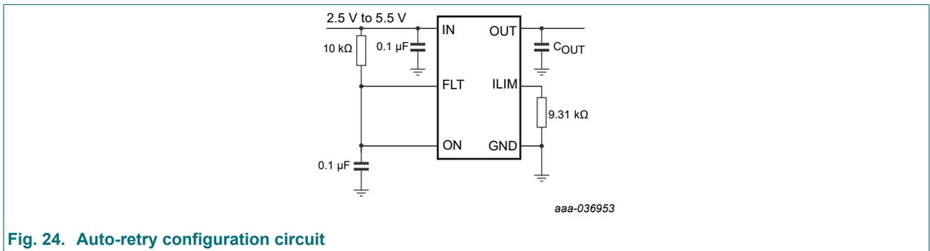
Fig. 24. Auto-retry configuration circuit
