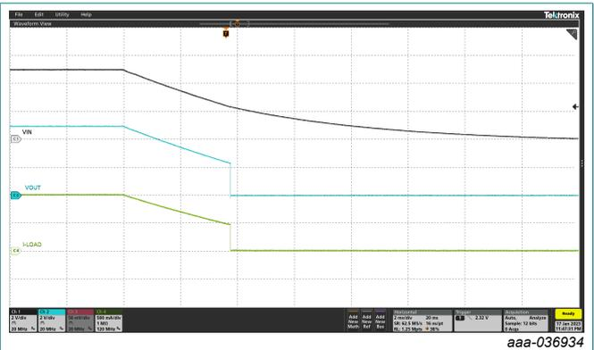
V<sub>IN</sub>=5 V, C<sub>OUT</sub> = 1 μF, R<sub>LIM</sub> = 20 KΩ, I<sub>load</sub> = 1 A
