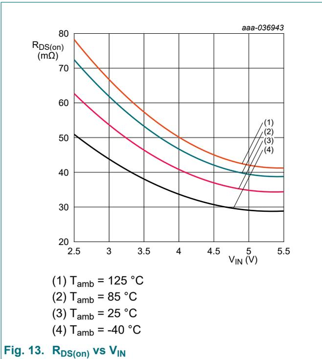
Fig. 13.  $R_{DS(on)}$  vs  $V_{IN}$
