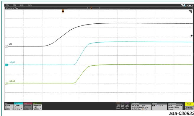
V<sub>IN</sub>=5 V, C<sub>OUT</sub> = 1 μF, R<sub>LIM</sub> = 20 KΩ, I<sub>load</sub> = 1 A
