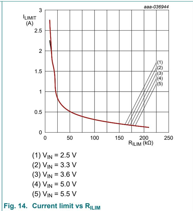
Fig. 14. Current limit vs  $R_{ILIM}$
