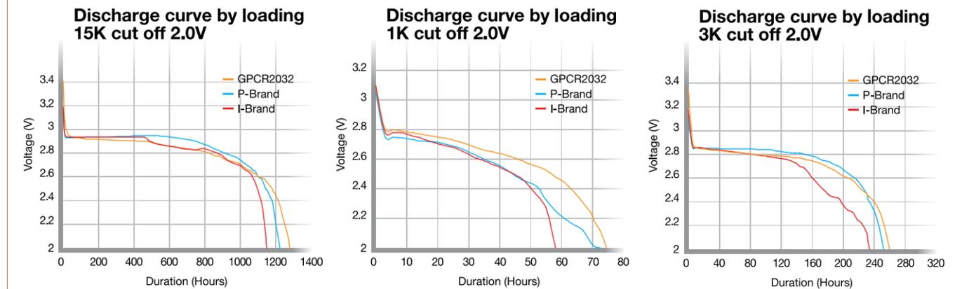
**GPCR2032 provides longer operating hours at different loading discharges.**
