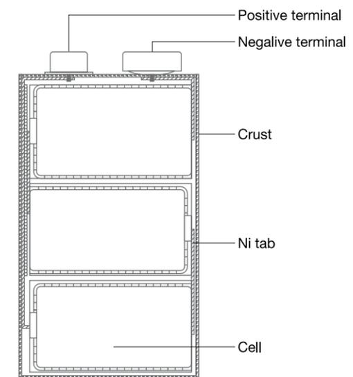
Cross sectional drawing of GP Primary Lithium Coin Batteries
