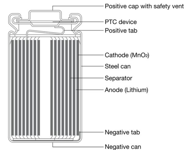
GP Primary Lithium 9V battery (GPCR-V9) is consisted of 3 pieces of GP Primary Lithium Cylindrical Batteries (GPCR14250)
