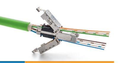
TE Connectivity's latest Industrial IP20 RJ45 Cat. 6<sub>A</sub> plug is based upon "common core" technology, a platform technology used in the entire industrial RJ45 product family. This RJ45 Cat. 6, plug is extending the family of Field Installable Cat5, common core designs with a connector that can be terminated tool-less with Cat6, cables in the field.
