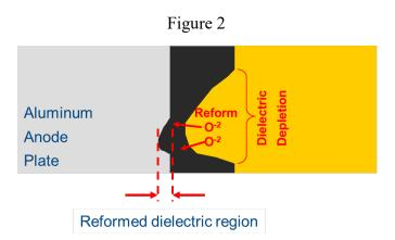
Leaving the capacitor unpowered for long amounts of time is not ideal because the selfhealing process can only take place when power is applied to the part. If the capacitor has been left unpowered for too long, and is then powered, the reforming process will occur much too rapidly. Large amounts of hydrogen gas will build up within the body of the part and cause the can to rupture.
