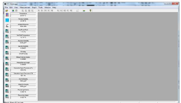
Now click on the thermometer icon and the icon with the water drops in the left side panel. The corresponding measuring curves are displayed.
