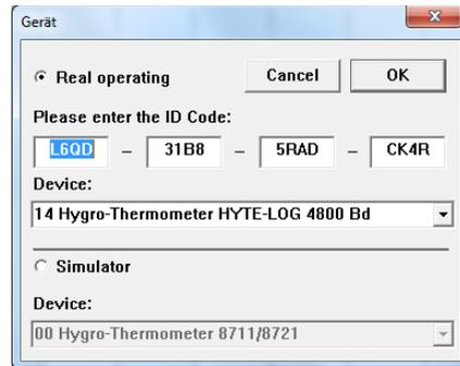
Now for the „Device“, select the device driver „14 Hygro-Thermometer HYTE-LOG 4800 Bd“. The activation code will be registered automatically. Confirm the dialogue with ‚OK‘. Now open the option „Extras“ in the menu and then go to the sub-menu „Interface“. Put in the corresponding interface.
