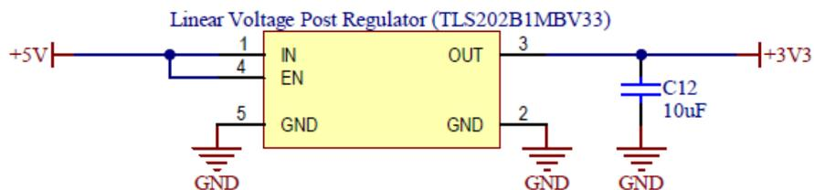
Figure 11 Infineon fixed linear voltage post regulator
