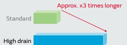
\*Pulse discharge condition: 45mA x 3s, 33s off, 2V cut off (23°C)
