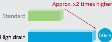
\*50% depth of discharge battery's maximum pulse discharge current over 2V for 3s (23°C)
