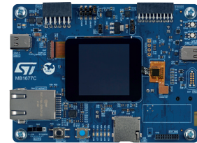
STM32H573I-DK* Multi connectivity kit USB, Ethernet, MicroSD, Display, 512-Mbit Octo-SPI flash, Audio, Multi-extension I/Fs, 176-pin MCU
