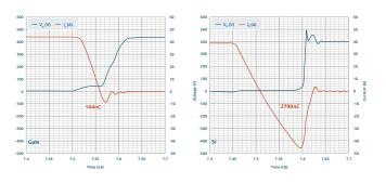
Figure 3 Qrr, Reverse recovery charges for GaN FET vs Si FET
