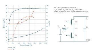
Figure 7 Half bridge boost converter (GaN switch vs Si CoolMOS
