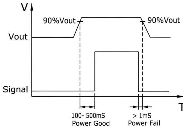
Figure 5. Power Good / Fail Signal Diagram
