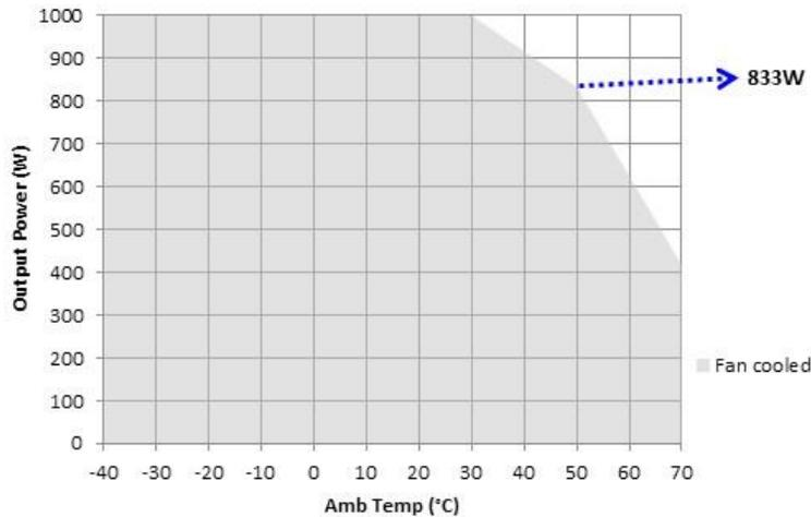
Figure 4. Power Derating Curve 24 V and above
