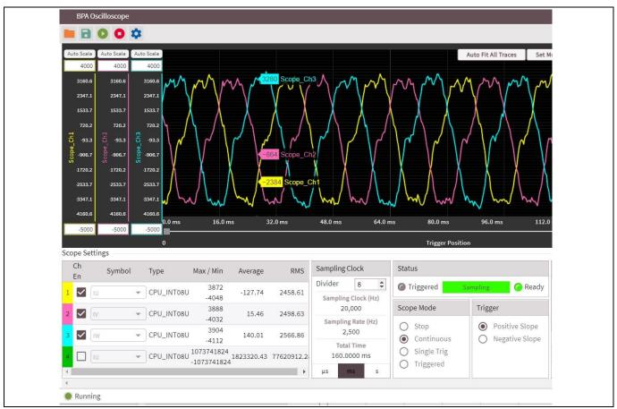
Figure 5 V/f open loop IU, IV, IW current waveform captured by the GUI's oscilloscope
