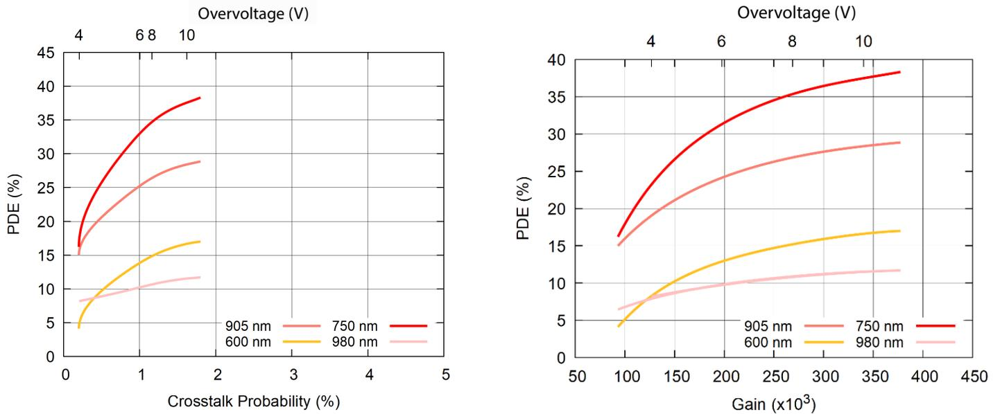
The AFBR-S4P11P012R combines high detection efficiency in the red and near infrared with very low crosstalk (<2%) and high dynamic range. This unique combination of electro-optical parameters makes this SiPM series an excellent device to boost system performance in a variety of applications, such as the following:
