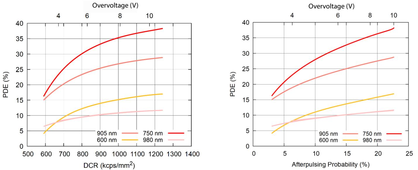
**Figure 4: PDE as a Function of the Dark Count Rate, Afterpulsing Probability, Crosstalk Probability, and Gain (Part 2)**
