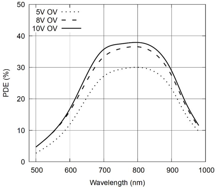
One implication of the wavelength dependency of the PDE saturation is that for two wavelength values with similar maximum absolute PDE but at different sides of the peak PDE, the overvoltage setting required to obtain the best signal-to-noise ratio might be different.
