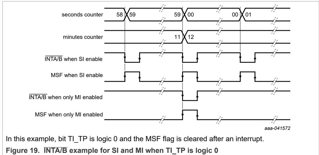
The pulse generator for the minute/second interrupt operates from an internal 64 Hz clock and generates a pulse of  $\frac{1}{64}$  seconds in duration.
