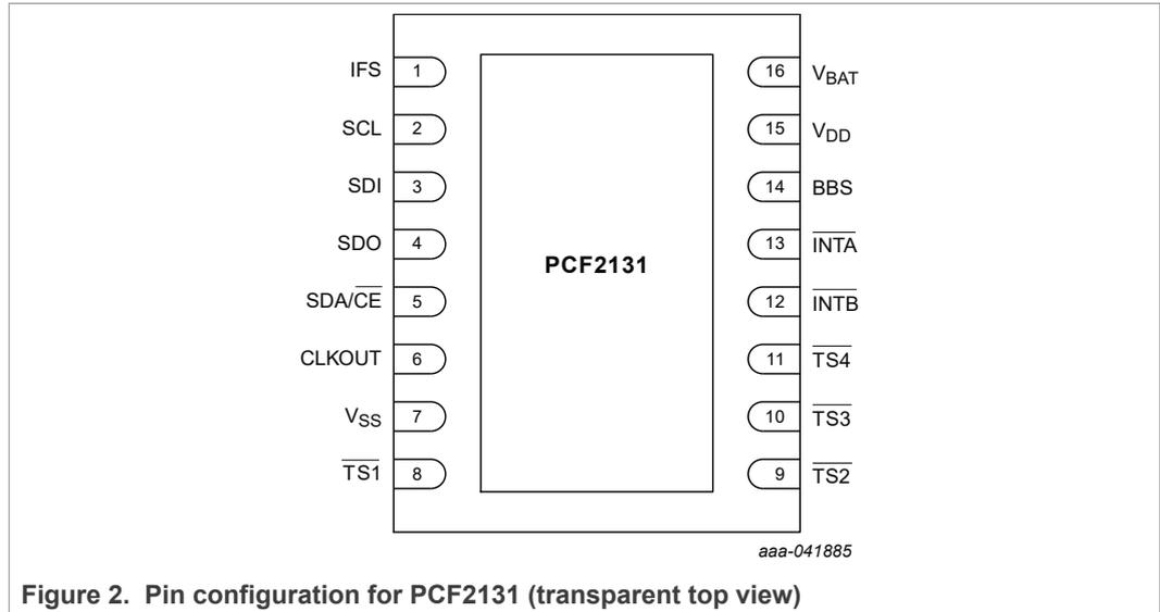
Figure 2. Pin configuration for PCF2131 (transparent top view)
