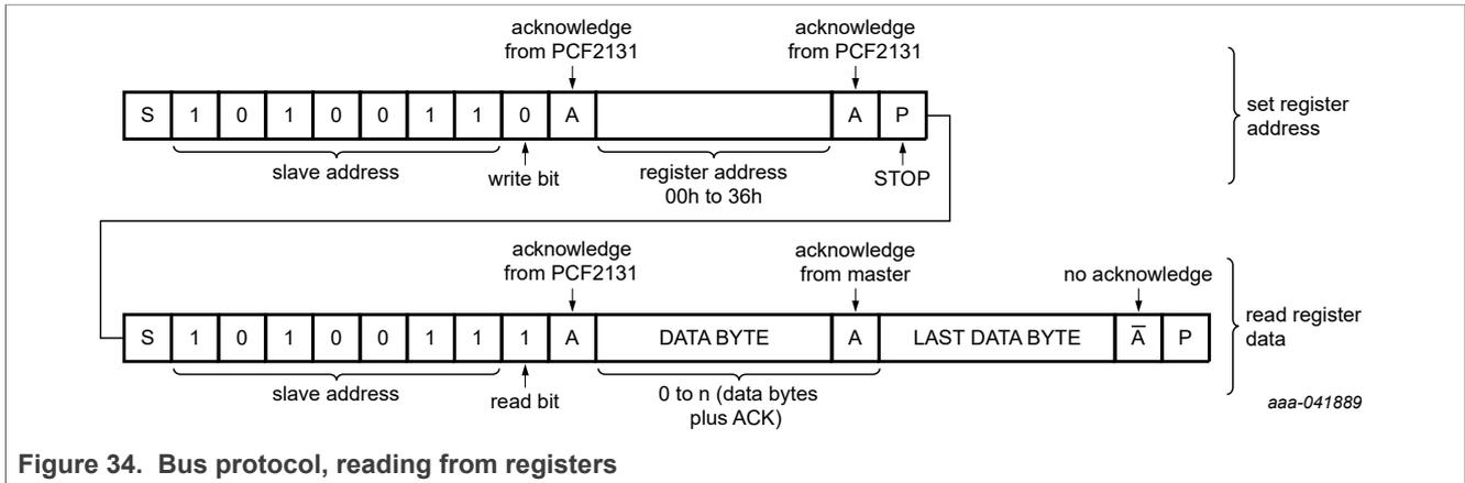
Figure 34. Bus protocol, reading from registers
