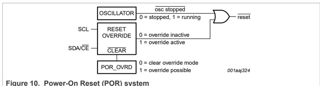
The setting of the PORO mode requires that POR\_OVRD in register Control\_1 is set logic 1 and that the signals at the interface pins SDA/CLE and SCL are toggled as illustrated in [Figure 11](#). All timings shown are required minimum.
