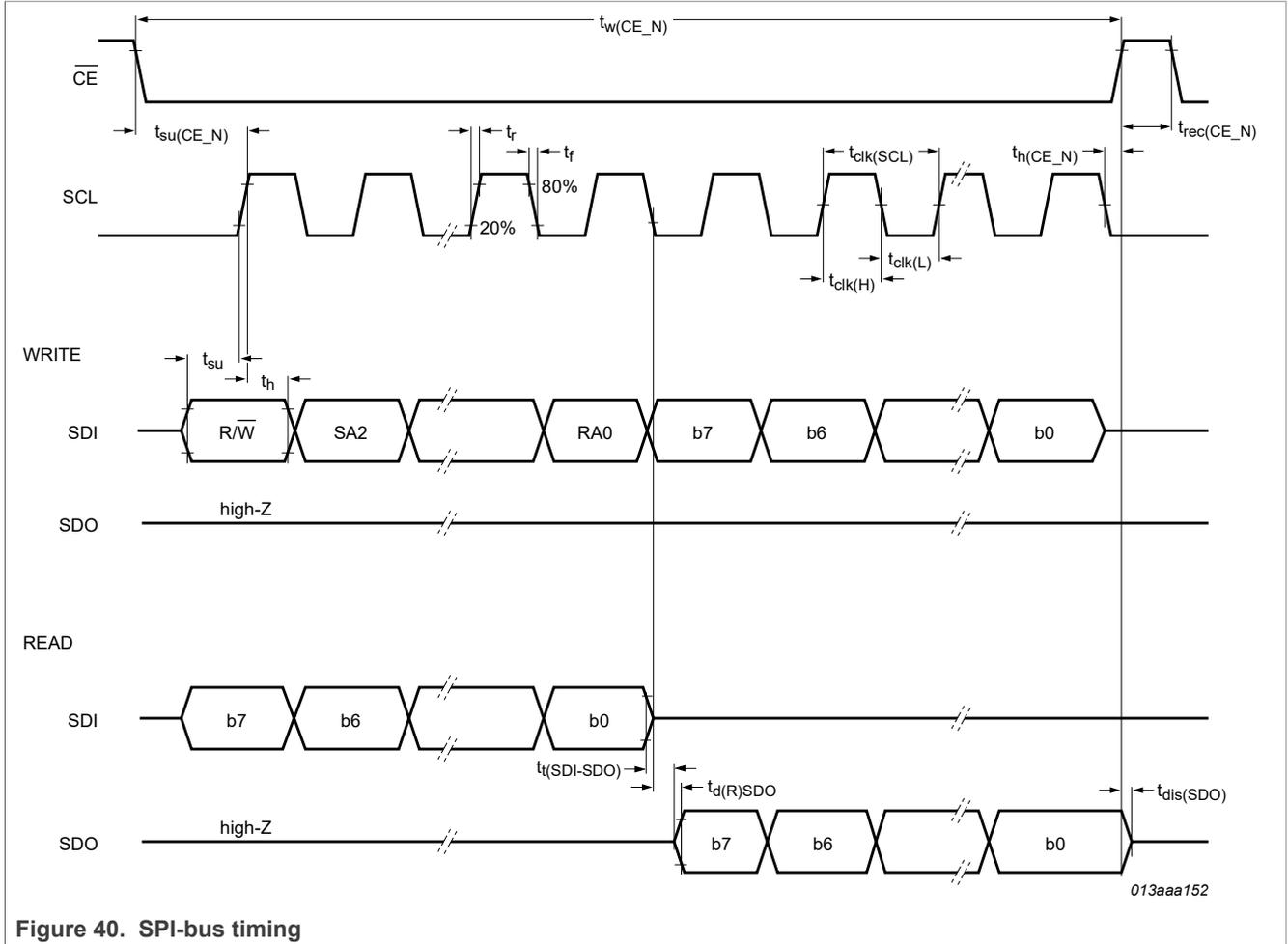
Figure 40. SPI-bus timing
