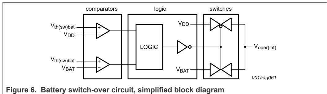
V<sub>oper(int)</sub> is at V<sub>DD</sub> or V<sub>BAT</sub> potential.
