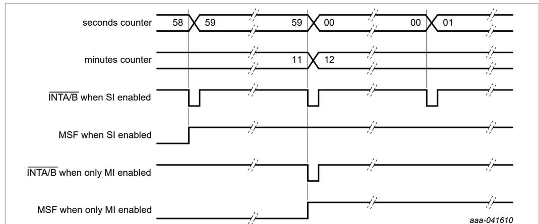
In this example, bit TI\_TP is logic 1 and the MSF flag is not cleared after an interrupt.
