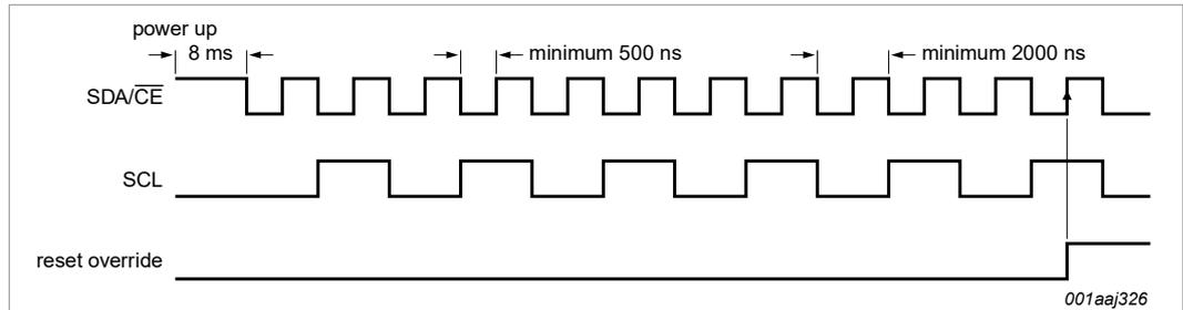
Figure 11. Power-On Reset Override (PORO) sequence, valid for both I<sup>2</sup>C-bus and SPI-bus
