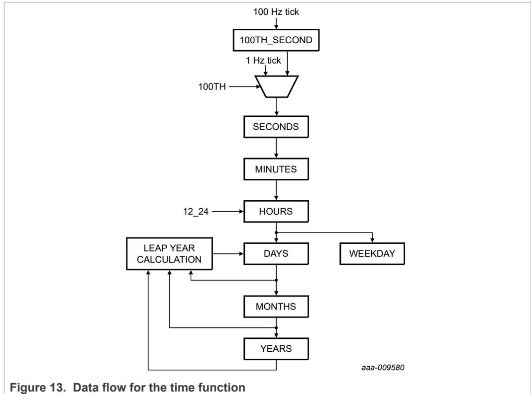
Figure 13. Data flow for the time function
