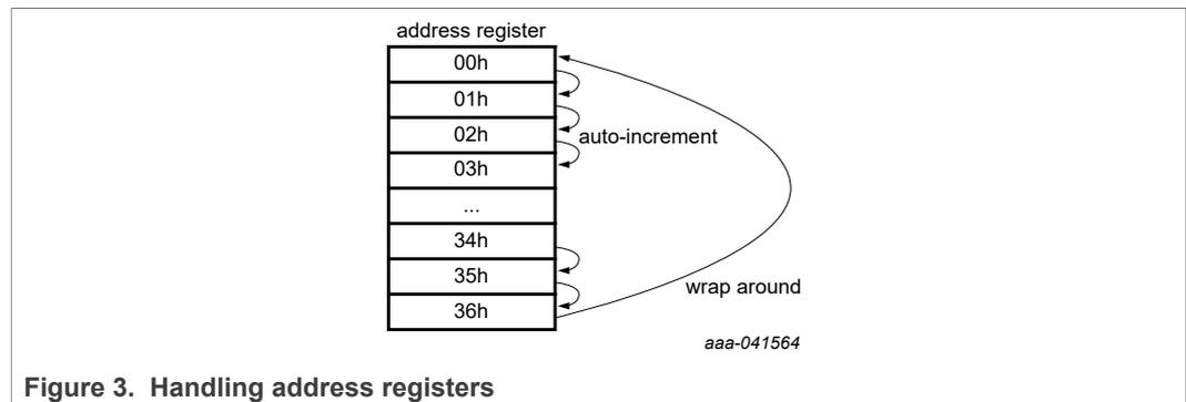
**Figure 3. Handling address registers**
