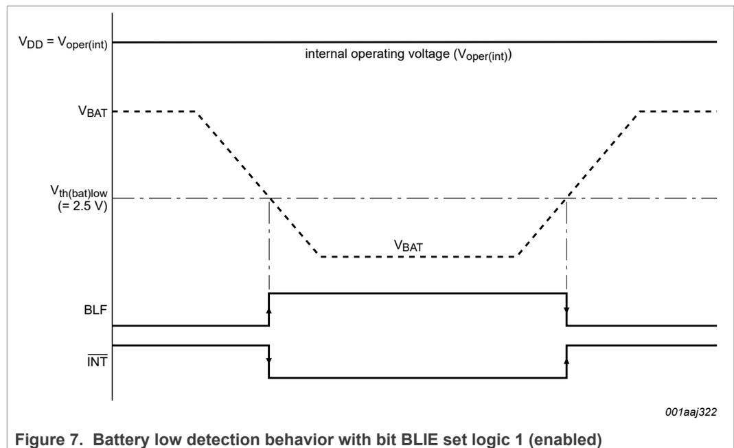
Figure 7. Battery low detection behavior with bit BLIE set logic 1 (enabled)
