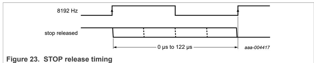
Figure 23. STOP release timing
