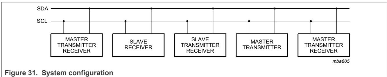
Figure 31. System configuration
