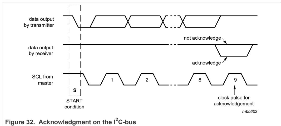
Figure 32. Acknowledgment on the I<sup>2</sup>C-bus
