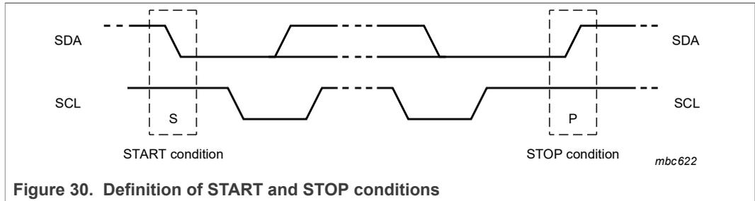
Figure 30. Definition of START and STOP conditions
