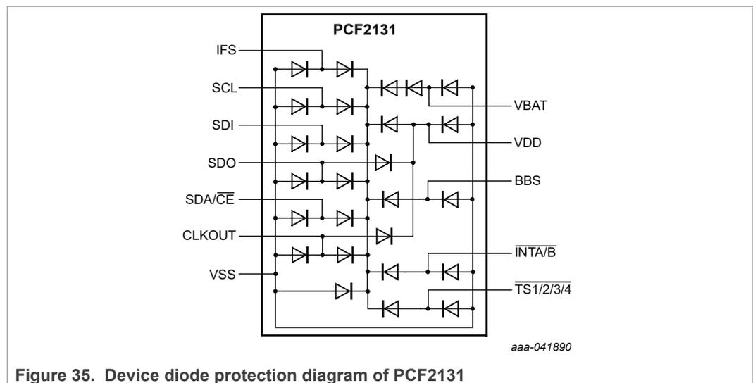
Figure 35. Device diode protection diagram of PCF2131
