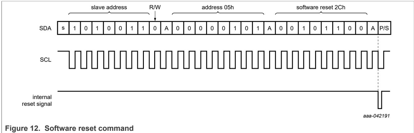
Figure 12. Software reset command
