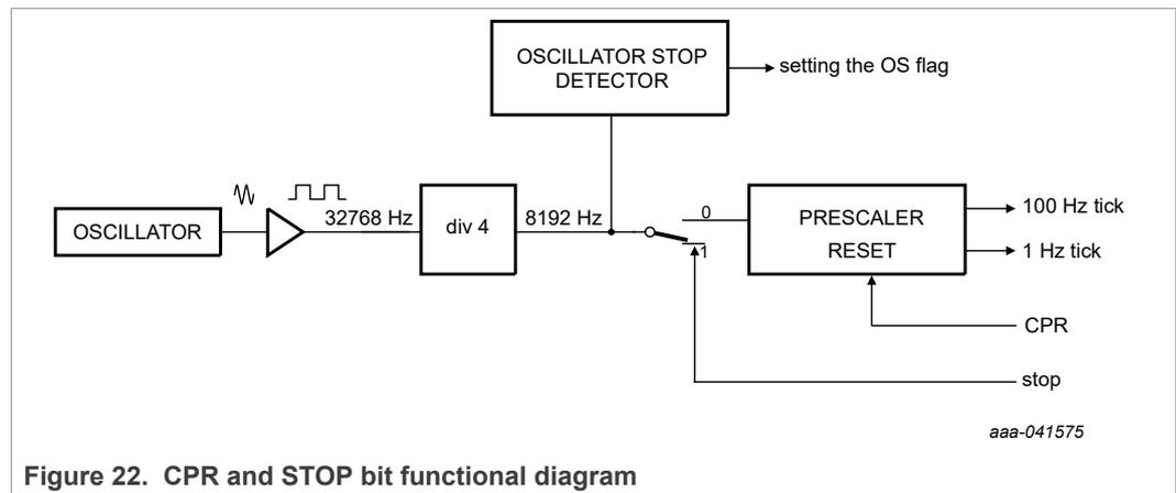
Figure 22. CPR and STOP bit functional diagram
