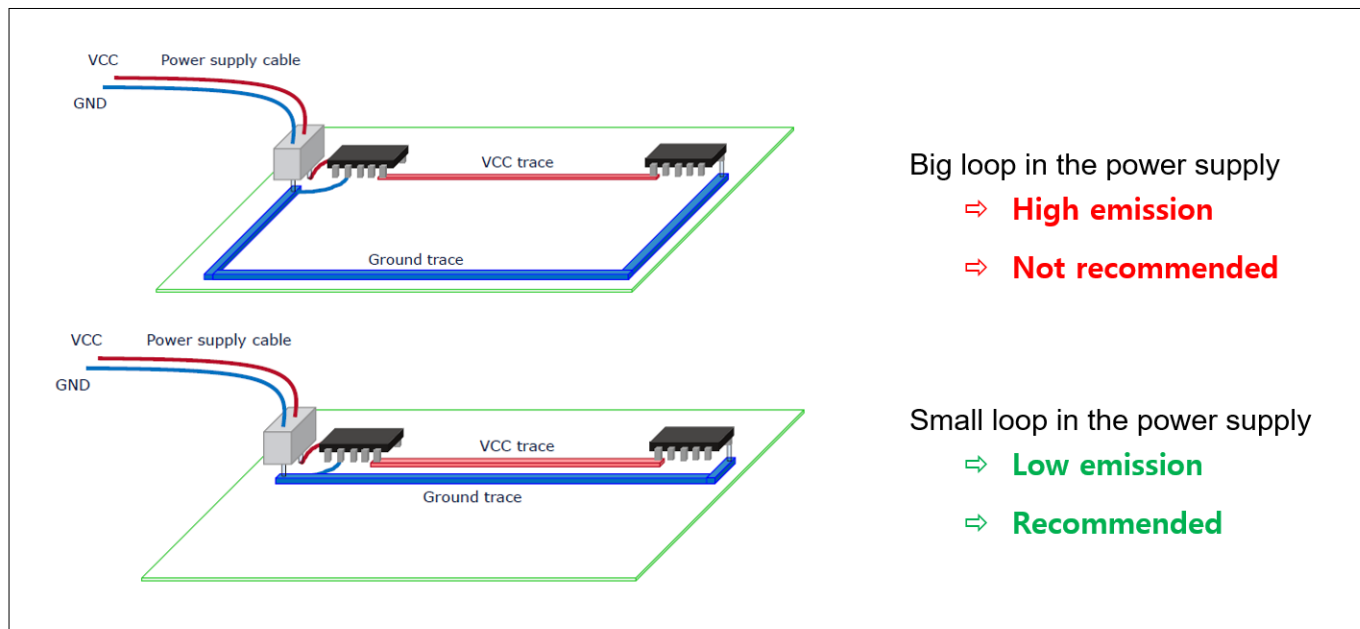
Figure 3 Routing of the power supply
