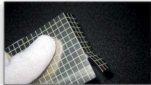
The Shield Can Kit <u>S01-806005KIT</u> allows you to make prototypes and limited quantities of cans, quickly and easily. The blanks are simple to cut and easy to form, requiring no special tooling. Pre-scored on a 5mm grid, cans of 5mm, 10mm or higher are possible. Maximum can size per sheet is 70mm x 50mm, 5mm high.
