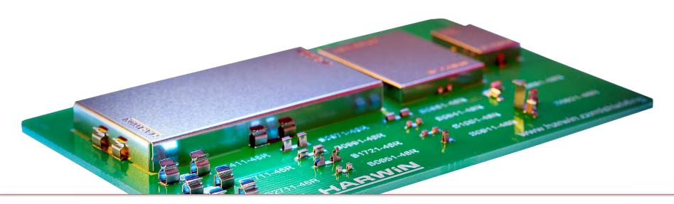
Harwin's SMT Clip and Can system works by soldering the Clips to the PCB during the SMT phase. The Cans are then pushed into the clips in a very quick secondary operation.
