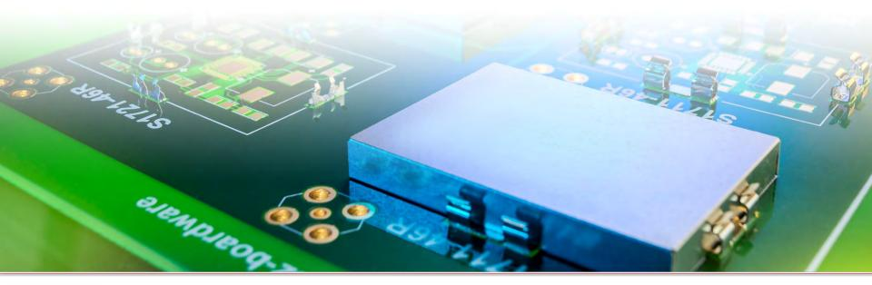
A soldered can that covers components requiring rework must first be desoldered. The remedial work underneath is carried out, then the can must be soldered back in place. Each solder operation adds the risk of damage, and greatly increases the rework cost due to time and operator skill.
