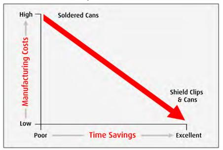
Removing the hand soldering phase and replacing it with a simple locate-and-press operation speeds up this secondary offline manufacturing process. Minimal skill is also required – it can even be automated with cans supplied in pick-and-place packaging. Costs are therefore saved on operator time and training – or eliminated completely.
