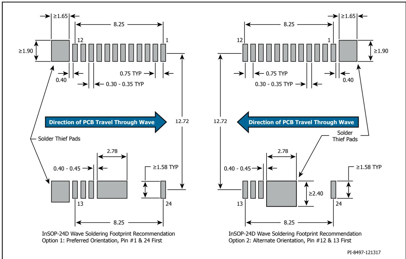
Figure 3. InSOP Wave Soldering Footprint Recommendations – Preferred and Alternate Orientations.
