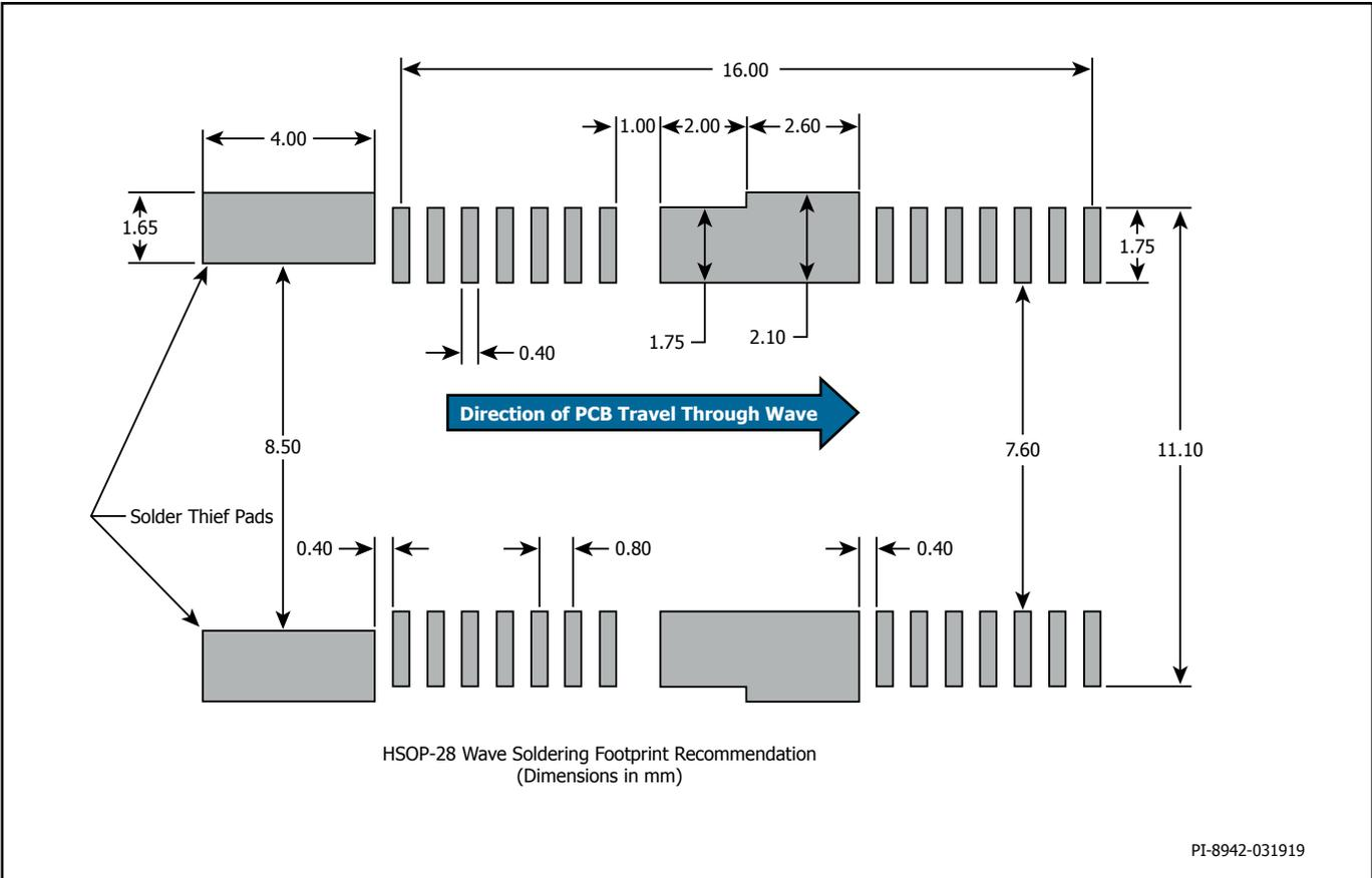
Figure 4. HSOP Wave Soldering Footprint Recommendation.
